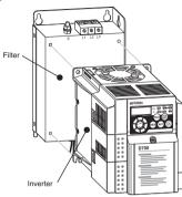
To fix the filter-inverter unit on the back of the cabinet use the mounting bolts provided with the filter. For correct filter performance the filter mounting bolts should electrically bond to the cabinet back panel wich is connected to earth. If this is not possible, the paint should be removed from the cabinet directly under the filter footprint
