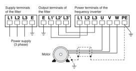
All cables must be shielded and earthed at both ends in order to reduce cable radiation. Earth motor, bond to filters.
