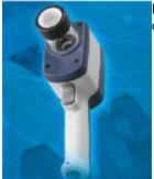
Lighting, lens, processing unit and interfaces are integrated in one device.
